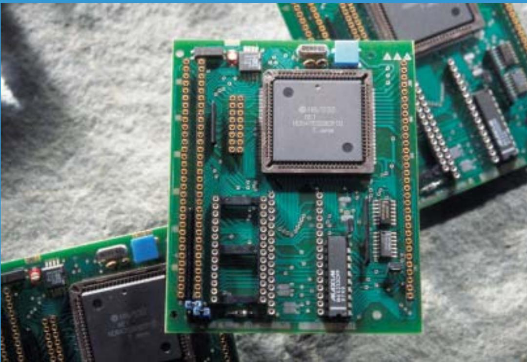
As a Data Collection Module with removable Card Memory option, you've little to add to its 10-bit 8-channel analog to digital converter, real time clock and memory of up to a gigabyte.
